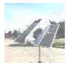
Energy Innovations - Standing over five feet square and five feet high, the Sunflower<sup>TM</sup> has 25 mirrors that track the sun, reflecting light onto the receiver. The solar cell array turns concentrated light into electricity while fans keep operating temperatures low. Cost is about two-thirds that of comparably rated PV-based systems. http://www.energyinnovations.com/
